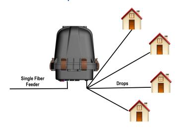
**Example Above:** Single fiber feeder with SC/APC 1x4 splitter and 4 SC/APC drops.
