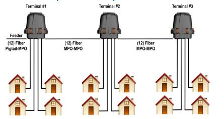
Example above: 12 fiber MPO feeder with 4 SC/APC drops and remaining fibers expressed out
