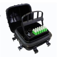
Ducts are simply brought to the YOURx-Terminal, trimmed to length and pushed into the YOURx FlexPorts on the base of the terminal - completing the protected pathway. Fiber is now pulled or pushed from the customer premise to the "inside" of the YOURx-Terminal, where the connector assembly is completed and mated.
