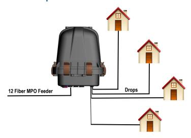
Example Above: 12 fiber MPO feeder with 4 SC/APC drops.
