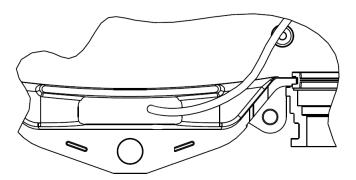
A cable exit is located at the bottom of the TAP Box which provides covered access to the inside of the building the box is mounted to.
