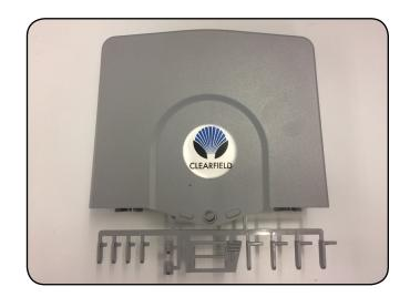
TAP Box will appear as shown. You will need a side cutters or pair of snips to remove the molded plastic pieces attached at the base of the box.
