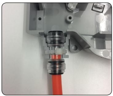
If not utilizing a coupler, cut two perpendicular slits in the center of the black cable entrance plug, and feed the cable through the plug. Then wrap the cable with grommet tape (foam tape) below the plug and secure it into place on the TAP Box with a zip tie. Insert the plug into place on the TAP just above.
