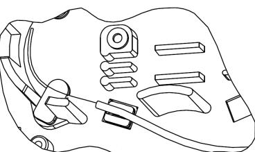
Cable tie downs, attached via VHB tape, can be used to secure the fiber prior to splicing.
