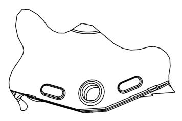
The TAP can be secured with either a lock or a security tab through the hole at the front of the box.
