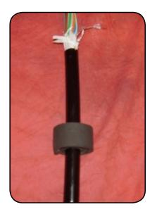
Place the foam gasket around the cable entrance hole in the bottom of the cabinet. Bring your cables up through the hole and slide them into the slots in feed through plate A.
