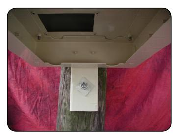
**Note:** Care should be taken to avoid over-tightening and deforming the hoist plate.
