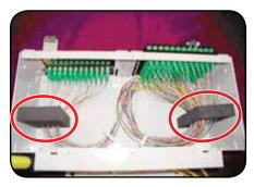
4. The 1RU panel will NOT have the separators and the 288 panel will have four separators (two will be stacked on top of each other on each side).
