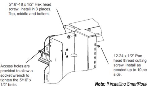
Note: Wait to tighten these 1/2" bolts until pan heads (10 per side) are installed
