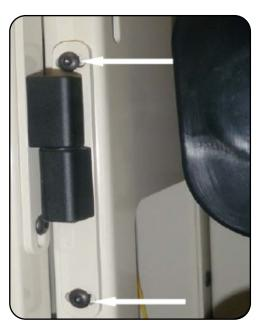
After the horizontal adjustments have been made, adjust the doors to be even vertically.
