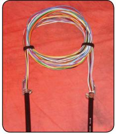
Ring cut/Mid-span opening
