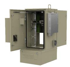
features an external AC Load Center. A door mounted integrated air-to-air heat exchanger and DC-powered fans cool the equipment inside the cabinet. A separate, vented, under-cabinet compartment houses optional batteries. A second battery compartment can be added for additional backup capabilities.
