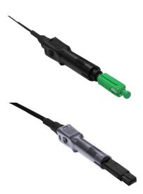
SeeChange Hardened Fiber Assemblies meet Clearfield's FiberDeep performance levels for low insertion loss (0.2dB max IL for single fiber and 0.35 max IL for MPO assemblies). Rigorous carrier grade testing has been performed on both connector styles ensuring optimal system performance long into the future.
