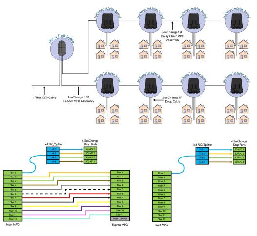
MPO Splitter Drop and Express Terminal Wiring Diagram MPO Splitter Drop Terminal Wiring Diagram
