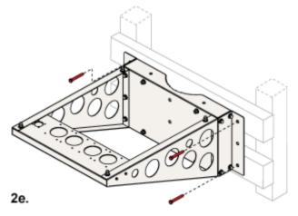
e. Install the appropriate user-supplied mounting hardware into the pilot holes to attach the bracket to the wall or frame. For example, use 1/2-inch lag screws for wood walls or H-frames, or concrete anchors for brick or stone walls.
