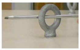
**2.** Using the Clearfield-supplied telco hex key, install a button-head Allen bolt into the vacant bolt hole.
