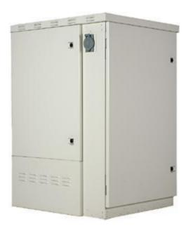
The ODC-1000 cabinet supports high density fiber and copper plant terminations, enabling deployment of a broad suite of applications from a single node. The cabinet's main electronics compartment is equipped with 23-inch front and rear equipment racks that provide a total of 36 RU of mounting space. The ODC-1000 typically houses one Calix C7 shelf, serving up to 480 copper access lines or up to 4096 PON subscribers.
