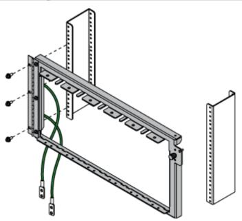
c. When the mounting frame is aligned correctly, secure the hinge side to the left rack using (3) self-tapping screws.
