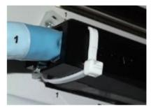
**Note:** To provide a securely-mated connection, be sure to align the head of the cable tie along the bottom edge of the RJ-21 connector as shown. Failure to install the cable tie correctly may result in an inadequate connection.
