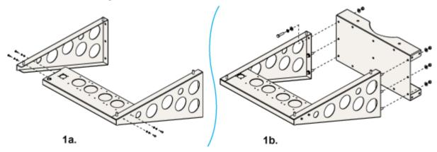
a. Attach the left and right support brackets to the cable entry bracket using (4) 1/4-inch hex head screws, (4) flat washers, (4) lock washers, and (4) nuts (two sets per side).
