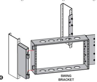
**4.** Attach the swing bracket to the left bracket by lowering its hinge channels onto the hinge posts.
