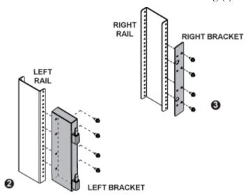
**3.** Install the right bracket onto the right rack rail using (4) self-tapping screws.
