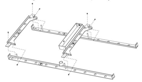
**6.** Tighten all screws to complete the template assembly.
