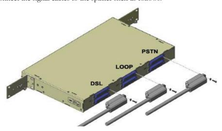
**Note:** Mating a CAT5 cable to the 90-degree CAT3 connector on the splitter shelf requires special attention, as only one side of the connector can be secured with a screw. The other side of the connector must be secured with a cable tie. The head of the cable tie must align with the bottom edge of the connector to achieve a robust connection. When supplying your own cables, Clearfield recommends using CAT5 cables to achieve optimal SNR margins.
