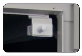
Note: Do not rotate the switch plunger. Rotating the plunger may damage the switch.
