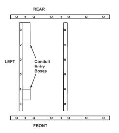
**Step 3:** Attach the short and long brackets together using eight supplied screws and nuts, as shown.
