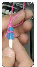
Note: You can secure more than one jumper to the fiber pull (for example, stagger and tape jumper connectors on the fiber pull).
