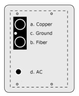
For proper cable entry into the cabinet, place conduit into the following locations.
