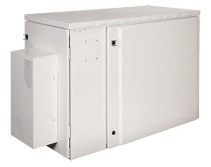
The base FAC 900 cabinet has a single compartment that houses electronics equipment together with high density fiber and copper plant terminations, enabling deployment of a broad suite of applications from a single node. The electronics area is equipped with a vertically-oriented 19-inch equipment rack that provides 8RU of mounting space.
