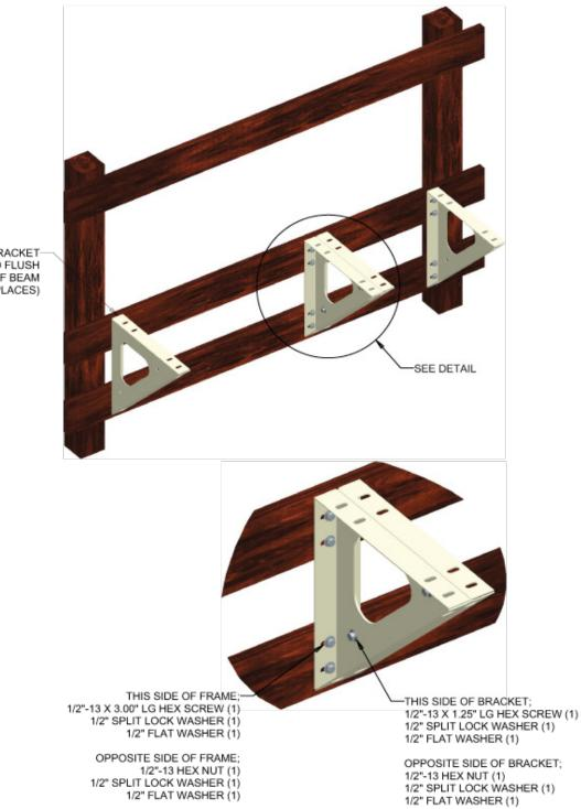
TOP OF BRACKET-MOUNTED FLUSH TO TOP OF BEAM (4-PLACES)
