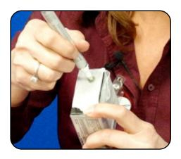
Lightly touch short side of the MTP/MPO Connector Swab to the wetted area (3-5 secs) to absorb some cleaning solution (DO NOT over saturate the swab).
