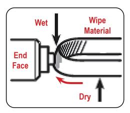
• Insert connector or insert probe though adapter and click 2-3 times to move past the wet area and allow material to dry wipe.
