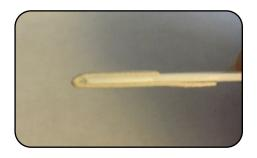
Wipe connector areas to be cleaned, sliding pad from bottom of pad across and forward to tip of swab, from 1 side to the other, turn over and use long side to dry in same movement.
