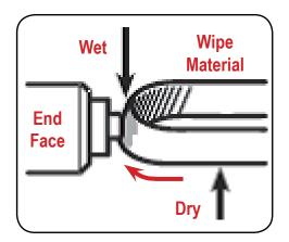
Insert connector or insert probe though adapter and click 2-3 times to move past the wet area and allow material to dry wipe.
