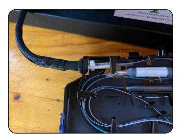
**3.** Bring split snakeskin wrap up and over the rubber strain relief boot, and tape it into place.
