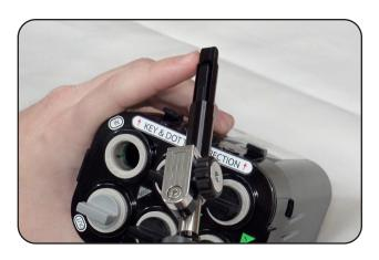
**2.** Scope the MPO port, and if necessary, proceed to cleaning.
