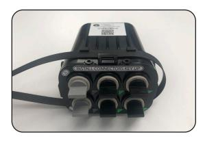
Insert each end of the strap through the holes on the outside of the spacer, directing the straps towards the center.
