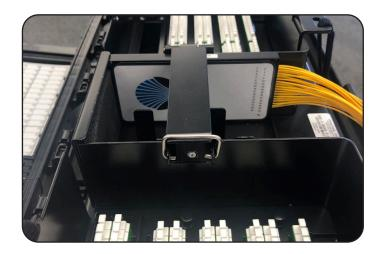
3. Route the splitter legs around to the side in which they will be connected. Utilize the velcro loops to hold the splitter legs in place.
