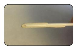
Wipe connector areas to be cleaned, sliding pad from bottom of pad across and forward to tip of swab, from 1 side to the other, turn over and use long side to dry in same movement.
