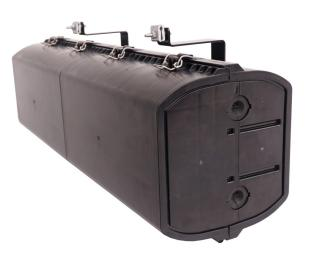
1. If needed, adjust the height of the mounting brackets on the Aerial FDH. The slotted holes in the mounting brackets will allow them to be installed at varying positions, and if needed you can remove the nuts holding the brackets to the case, and choose the new holes which best fit your needs. Secure the brackets back to the case with a can wrench.
