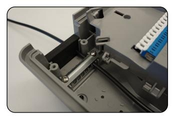
**8.** Reinstall the cable retention grommet plate, securing it in place with the two screws.
