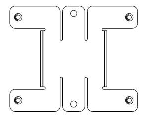
When installing the mounting bracket onto a metal pole, utilize a band clamp. The clamp will slip through the slot in the underside of the mounting bracket. Once the clamp is through the mounting bracket, secure the bracket to the pole using the band clamp.
