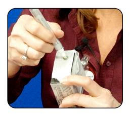
Lightly touch short side of the MTP/MPO Connector Swab to the wetted area (3-5 secs) to absorb some cleaning solution (DO NOT over saturate the swab).
